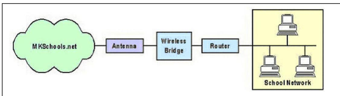
*(In three instances where there is no line of sight between a core site and a school, a DSL connection through phone lines has been used)*
